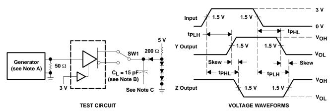
NOTES: A. The input pulse is supplied by a generator having the following characteristics:  $t_f \le 5$  ns,  $t_f \le 5$  ns, PRR  $\le 1$  MHz, duty cycle = 50%,  $Z_O = 50 \Omega$ .
